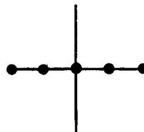
$$\frac{\partial^4 f_{0,0}}{\partial x^4} = \frac{1}{h^4} (f_{2,0} - 4f_{1,0} + 6f_{0,0} - 4f_{-1,0} + f_{-2,0}) + O(h^4)$$
