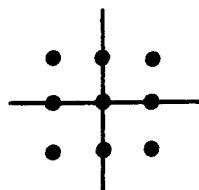
$$\begin{aligned} \frac{\partial^4 f_{0,0}}{\partial x^2 \partial y^2} = & \frac{1}{h^4} (f_{1,1} + f_{-1,1} + f_{1,-1} + f_{-1,-1} \\ & - 2f_{1,0} - 2f_{-1,0} - 2f_{0,1} - 2f_{0,-1} + 4f_{0,0}) + O(h^2) \end{aligned}$$
