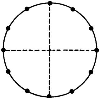
$$\frac{1}{2\pi h} \int_{\Gamma} f(x, y) ds = \frac{1}{2m} \sum_{n=1}^{2m} f\left(h \cos \frac{\pi n}{m}, h \sin \frac{\pi n}{m}\right) \\ + O(h^{2m-2})$$
