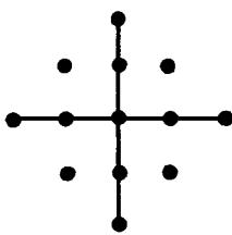
$$\nabla^4 u_{0,0} = \left( \frac{\partial^4 u}{\partial x^4} + 2 \frac{\partial^4 u}{\partial x^2 \partial y^2} + \frac{\partial^4 u}{\partial y^4} \right)_{0,0}$$
