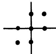
$$\begin{aligned} \frac{\partial^2 f_{0,0}}{\partial x \partial y} = & \frac{-1}{2h^2} (f_{1,0} + f_{-1,0} + f_{0,1} + f_{0,-1} \\ & - 2f_{0,0} - f_{1,1} - f_{-1,-1}) + O(h^2) \end{aligned}$$
