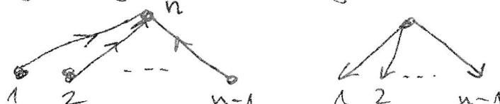
$$\begin{aligned} \text{Broj poruka} &= 2n-2 \\ \Rightarrow \text{mbp}(n) &= 2n-2. \end{aligned}$$
